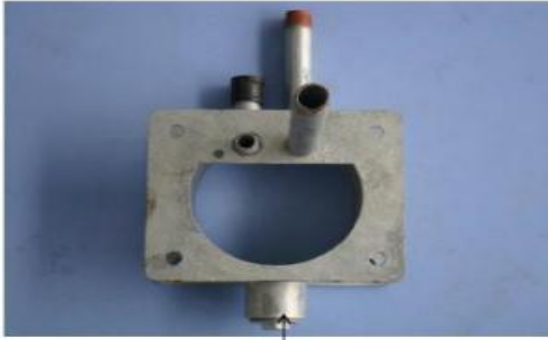
Inlet for rooftop rainwater harvesting
